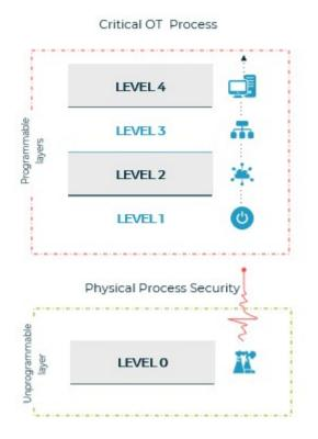
Process-oriented OT cybersecurity integrates **real-time monitoring** of Level 0 data to identify threats that may not be visible at the higher levels. By continuously analyzing operational parameters and comparing them to baseline conditions, this approach enables organizations to detect anomalies indicative of malicious activity. For example:
