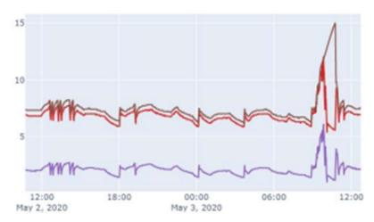
Normal chiller temperature as compared to the anomaly that was detected. The anomaly was caused by a power outage which raised the temperatures of the chilled water.
