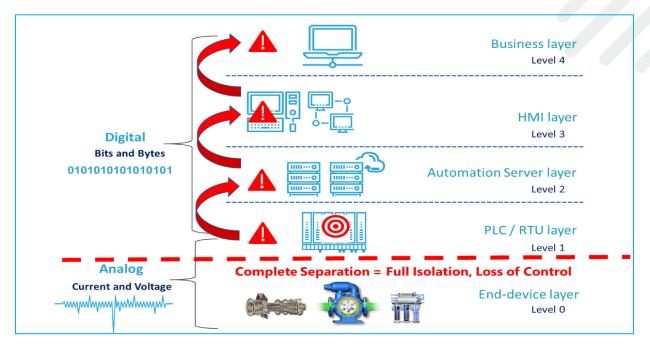
An attacker has taken control of a critical process while a perfectly normal operational status is reflected on the HMI and other levels. The attack is allowed to continue undetected because the control system's Level 1 (and above) monitoring devices are blind to what is happening at Level 0 (the physical layer).
