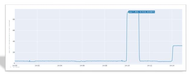
2. The AD tool detects this process anomaly at 14:09:50 (immediately) with various ML models (TCM and TCM with states models). Alert is fired in the GUI and sent by e-mail to Iren's team. The users can now see the alert details and visualization of the attack on the sub-station process.
