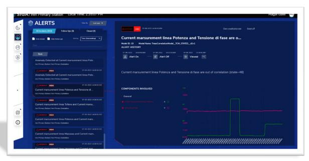
3. The user enters the ML visualization tool in the GUI to investigate the alert and understand where, how and when the attack took place on the process. The following graph is a the TCM correlation map, presenting the correlation between the Potenza line and the bus bar voltage. The blue area is the normal behavior correlations area and the dots outside of it are the abnormal correlations from the attack.
