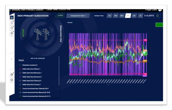
The AD tool GUI in the pilots is enabling the users full visualization of the process, receive alerts on anomalies, perform analysis and forensics etc.
