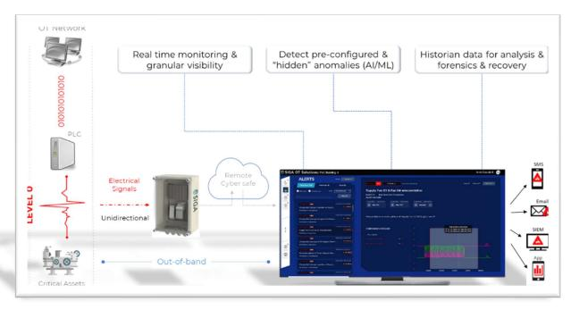
The AD tool is customized especially for the EPES market. It can be installed on level 0 of OT systems of all EPES utilities (generation, distribution etc.). With its new developed ML models, the tool can provide the EPES critical assets with level 0 process anomaly detection, that will enhance the ability to detect cyberattacks that are trying to compromise and intervene with the EPES machinery/process proper operation. The tool will detect the attack in its early stage and alert the operators
