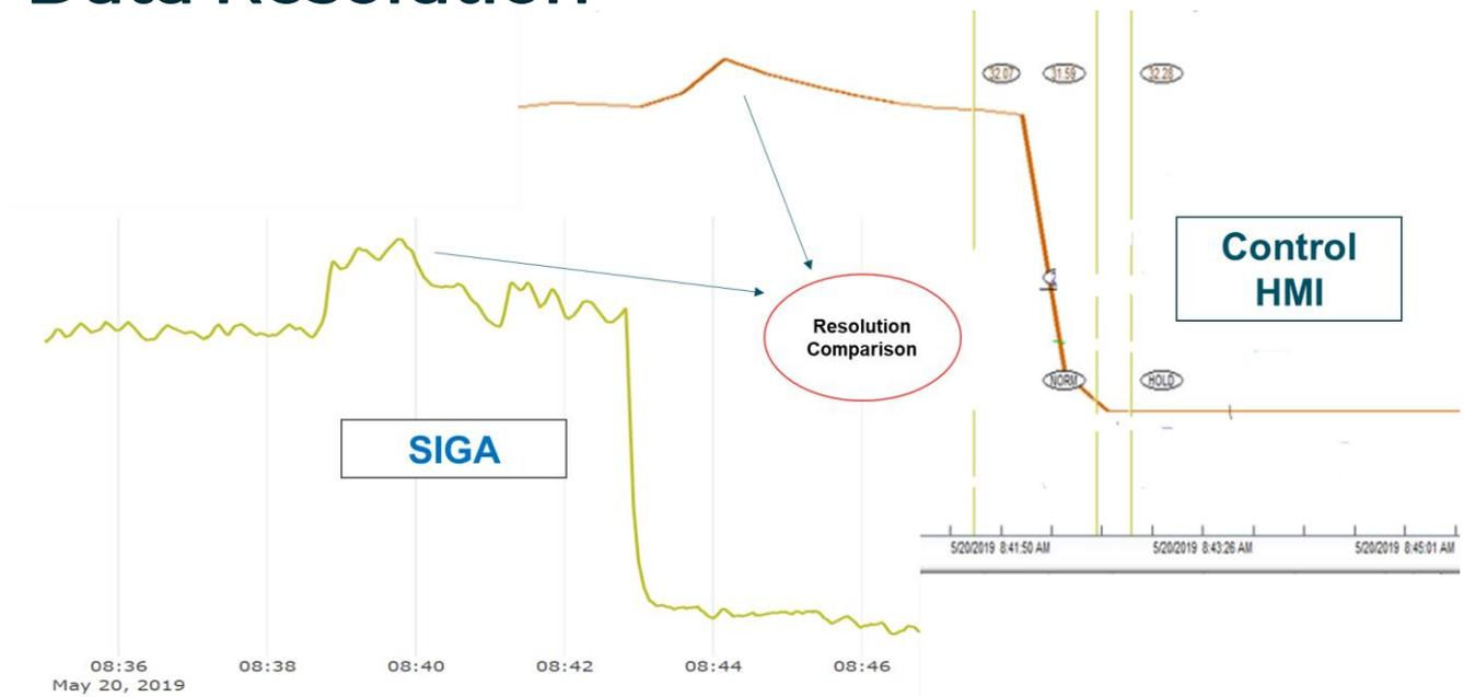
Comparing the SIGA graph to the control HMI graph showed unprecedented granularity into the process data
